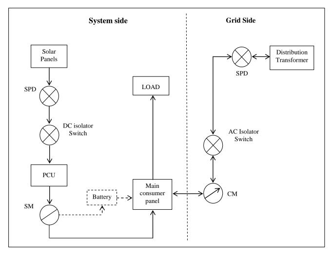
SPD- Surge Protective Device, PCU- Power Conditioning Unit, SM-Solar Generation Meter, CM- Consumer Meter (Net meter or Bi-directional meter)
