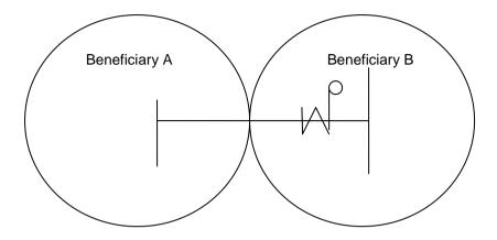
$\underline{\text{Case} - 2}$ : Interconnecting line owned by Beneficiary - B Metering point: Substation of Beneficiary-A
