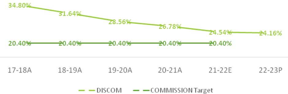
AT&C and Distribution loss have decreasing trend though approval is constant. The gap of approve and actual needs to reduce further and lower approval target is needed.
