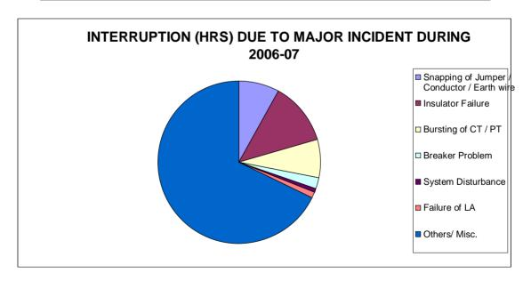
272. The Commission expresses grave concern about the interruptions occurring in the EHT transmission system due to snapping of conductors, burning of jumpers, failure of insulators, bursting of CTs/PTs, damage to transmission towers, failure of equipments at various sub-stations causing dislocation of power supply which can hardly be tolerated in view of growing importance for maintaining continuity and quality of power supply in the developing industrial economy of the State. Theft of
